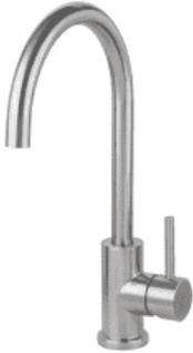
This type of faucet currently has no requirement for which direction should be the hot supply. I am proposing that hot should be to the back or far side of the fixture to prevent scalding to small children. A child that can barely reach the controls will inherently pull the handle toward themselves. If this is the direction of the hot supply, it could lead to injury of the child.
